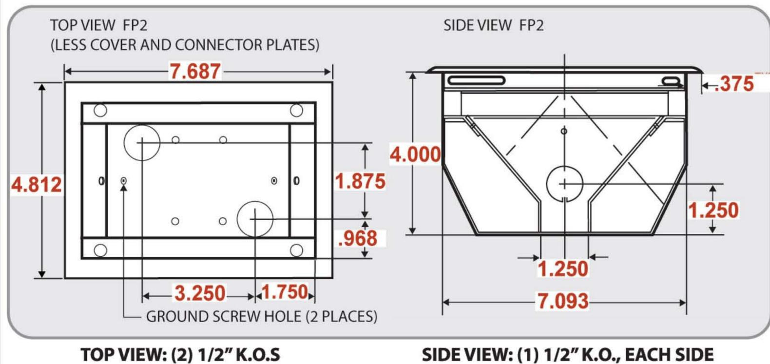
POCKET 5&8 HAVE "DOUBLE-KNOCKOUTS" For 1/2" & 3/4" CONDUIT. Total of 4 knock-outs, 1) on each side, 1) on the back, 1) on the bottom of the back
